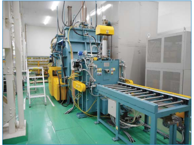
Vacuum Furnace with Computer Aided Precise Temperature Control
