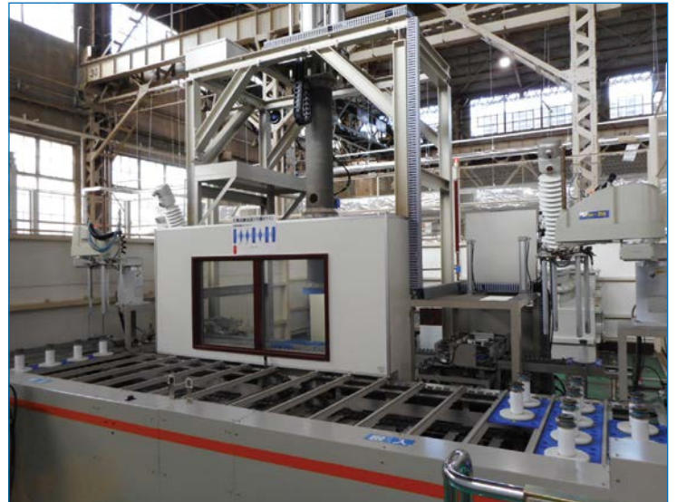
Automated Interrupter Testing Facility with Computer Aid
