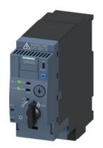
SIRIUS Compact load feeder DOL starter 690 V 110...240 V AC/DC 50...60 Hz 1...4 A IP20 Connection main circuit: plug-in, without terminals Connection auxiliary circuit: plug-in, without terminals
