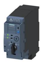
SIRIUS Compact load feeder DOL starter 690 V 24 V AC/DC 50...60 Hz 0.1...0.4 A IP20 Connection main circuit: plug-in, without terminals Connection auxiliary circuit: plug-in, without terminals
