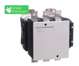
NEMA Contactor, TeSys N, nonreversing, Size 6, 540A, 400HP at 460VAC, 3 pole, 3 phase, 120VAC 50/60Hz coil, open
