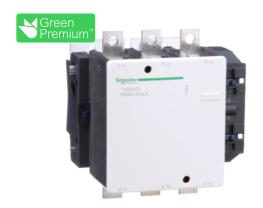
NEMA Contactor, TeSys N, nonreversing, Size 5, 270A, 200HP at 460VAC, 3 pole, 3 phase, 120VAC 50/60Hz coil, open
