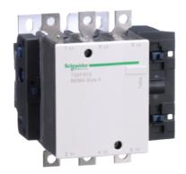
NEMA Contactor, TeSys N, nonreversing, Size 4, 135A, 100HP at 460VAC, 3 pole, 3 phase, 120VAC 50/60Hz coil, open
