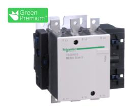
NEMA Contactor, TeSys N, nonreversing, Size 3, 90A, 50HP at 460VAC, 3 pole, 3 phase, 120VAC 50/60Hz coil, open
