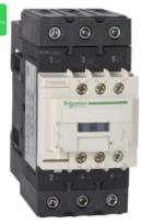
Contactor, Tesys N Contactors, nonreversing, NEMA size 2, 45A, 25HP at 460VAC, 3P, 3 phase, 24VDC coil, open
