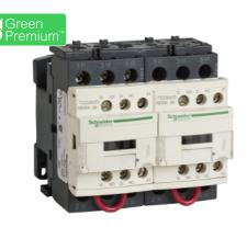
NEMA Contactor, TeSys N, reversing, Size 00, 9A, 2HP at 460VAC, 3 pole, 3 phase, 120VAC 50/60Hz coil, open
