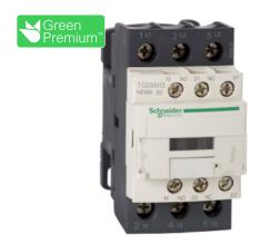
NEMA Contactor, TeSys N, nonreversing, Size 00, 9A, 2HP at 460VAC, 3 pole, 3 phase, 24VAC 50/60Hz coil, open
