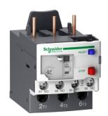
Thermal overload relay, TeSys Deca, 690VAC, 23 to 32A, 1NO+1NC, class 20, screw terminal, for unbalanced loads
