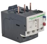
Thermal overload relay, TeSys Deca, 690VAC, 9 to 13A, 1NO+1NC, class 20, for unbalanced loads
