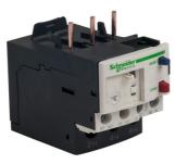
Thermal overload relay, TeSys Deca, 690VAC, 1.6 to 2.5A, 1NO+1NC, class 20, for unbalanced loads
