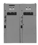
Switchgear, HVL switch, 600A, 15 kV, 3 pole, switched fuse mechanism, 10A to 400A E boric acid fuse, NEMA 3R
