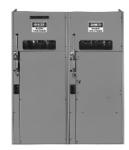
Switchgear, HVL switch, 600A, 15 kV, 3 pole, switched fuse mechanism, 10A to 400A E boric acid fuse, NEMA 1
