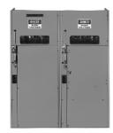
Switchgear, HVL switch, 600A, 4.76 kV, 3 pole, switched fuse mechanism, 10A to 450A E DIN/E current limit fuse, NEMA 3R
