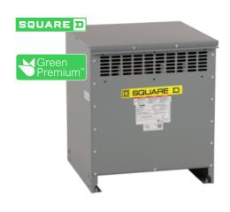
Low voltage transformer, DOE 2016, dry type, 3 phase, 45kVA, 480V pri, 208Y/120V sec, Cu, 80C rise, Type 2
