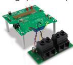
This is a fully functional single phase meter featuring the PIC18F87J72 MCU with Analog Front End. This low-cost design uses a shunt for the current sensor. The PIC18F87J72 drives the LCD and includes both an isolated USB and non-isolated RS232 interface for calibration
