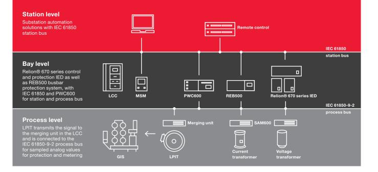
Hitachi Energy's world-leading digital substations, based on the international standard, IEC 61850, break benchmarks in regard to reliability, interoperability and realtime performance, thus bridging the gap between process bus and the station levels.
