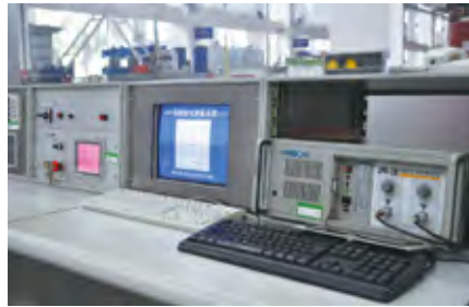
Transformer Load Loss Test System
