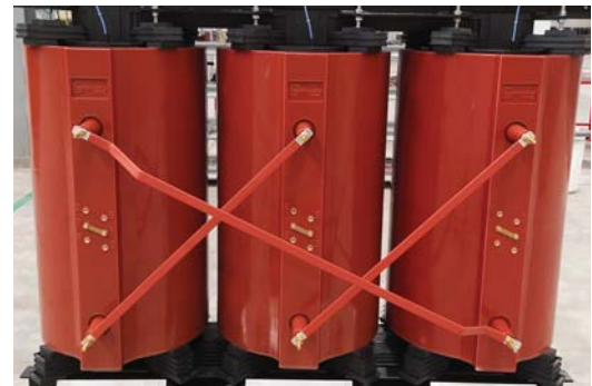
example of HV terminals
