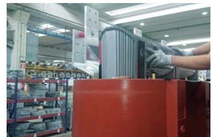
Core coils assembly
